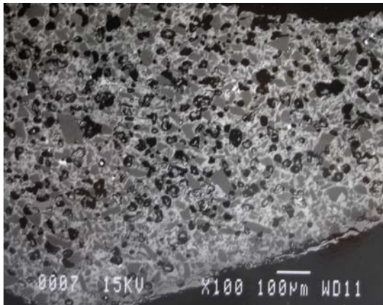
Faience in Ancient South Asia. Fig. 2 Backscattered electron image from a scanning electron microscope of a cross section of a faience bangle bracelet from Harappa. The dark gray grains are quartz, the light gray matrix is the glass phase. The exterior of the bangle runs along the lower edge of the photomicrograph and a thin glaze layer is visible along part of the length at the lower right.
